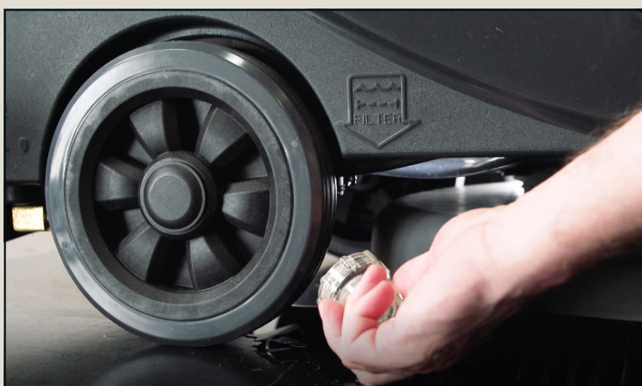
Check and clean the water filter (weekly)
