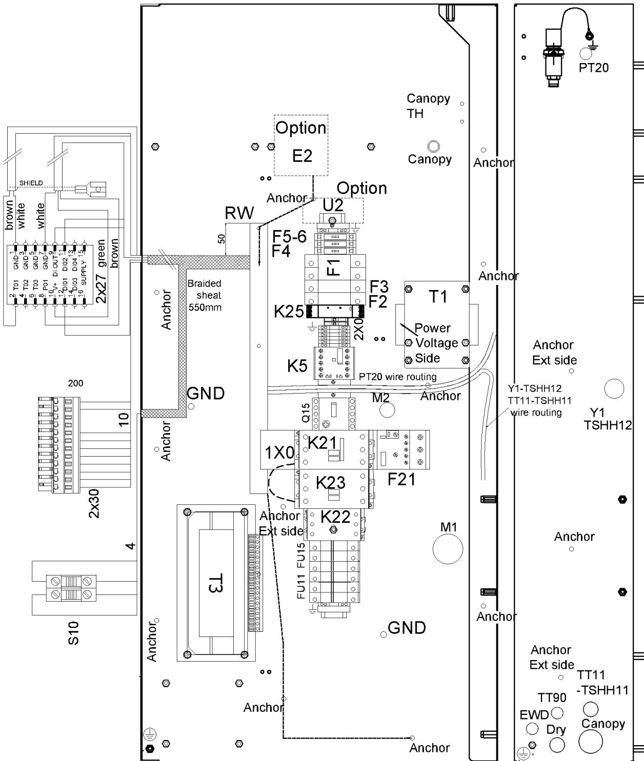
**42 - Cubicle components CPBg 20-34 - 575V/60Hz - Without dryer - Gear driven**
