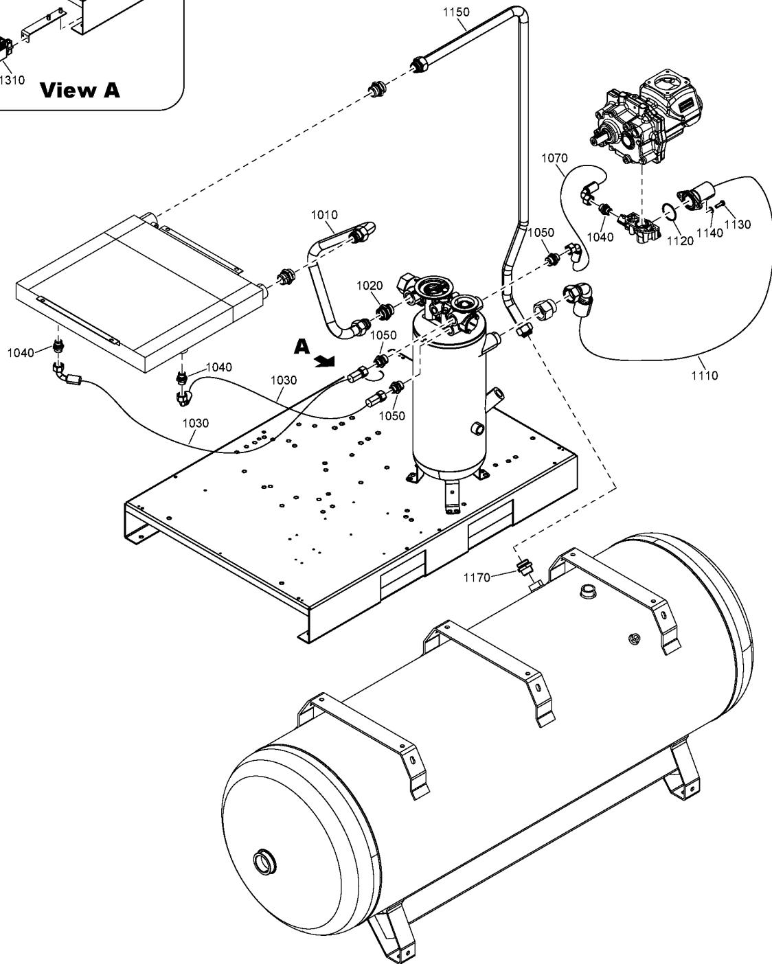
**17 - Air outlet CPB<sub>g</sub> 20, CPB<sub>g</sub> 25, CPV<sub>Sd</sub> 21, CPV<sub>Sd</sub> 25 - Tank-mounted - Without
