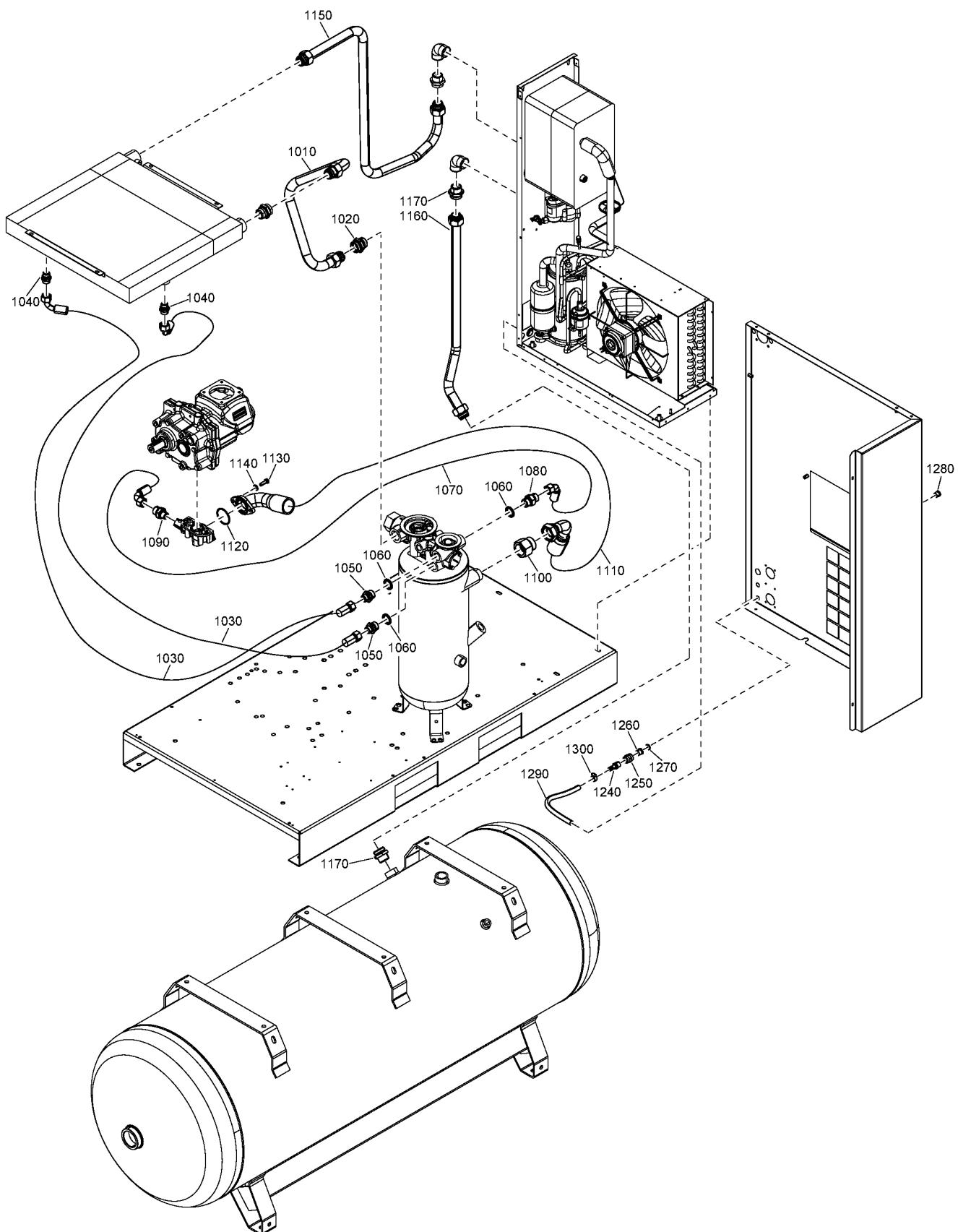
**24 - Air outlet CPBq 29, CPVSd 29 - Tank-mounted - With dryer**
