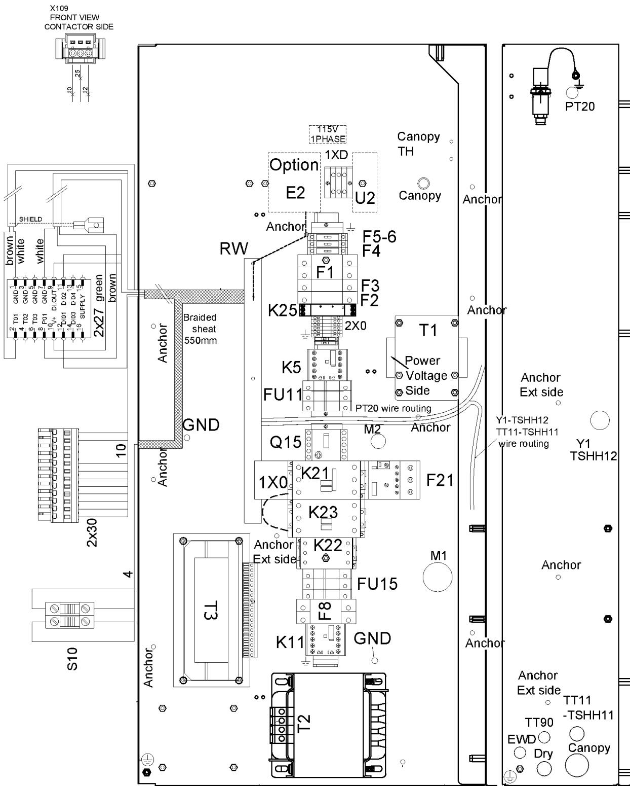
**43 - Cubicle components CPBg - 20-34 - 575V/60Hz - With dryer - Gear driven**
