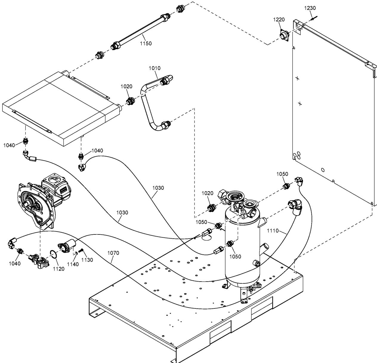
**14 - Air outlet CPBg 20, CPBg 25, CPVSD 21, CPVSD 25 - Floor-mounted - Without dryer**
