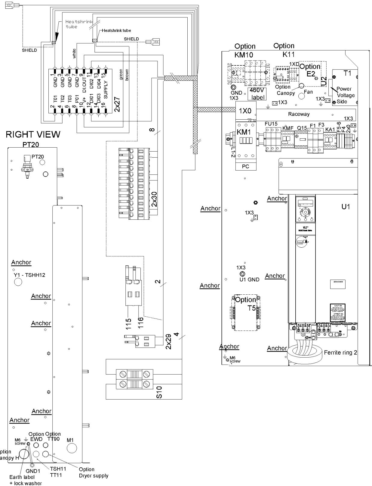
**47 - Cubicle components CPVSd 21-34 - 460V/60Hz - ASME, (CRNASME - Without dryer) - Direct driven**
