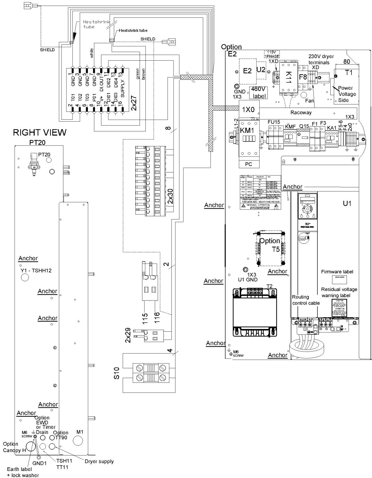
**48 - Cubicle components CPVSd 21-34 - 460V/60Hz - CRNASME - With dryer - Direct driven**
