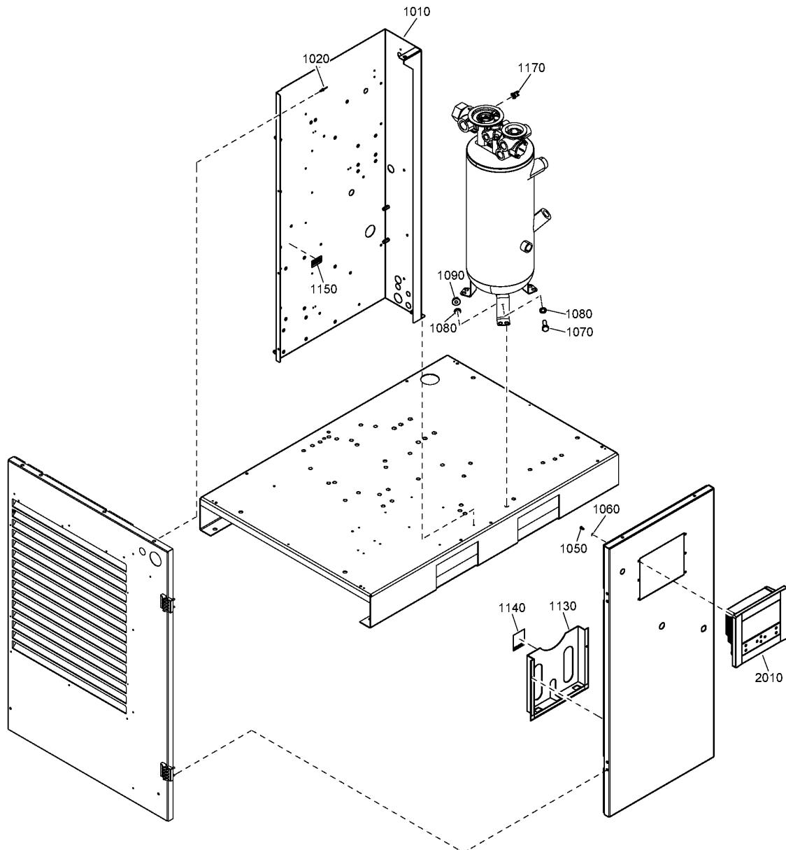
**32 - Regulation CPBg 20-34 - Gear driven – (AS1210, ASME, CE, MOM, SA – 400V), (CE – 230V), (ASME – 200230460V, 230V, 380V, 440V), (CRNASME – 575V), (CRNASME – 200230460V – With dryer)**
