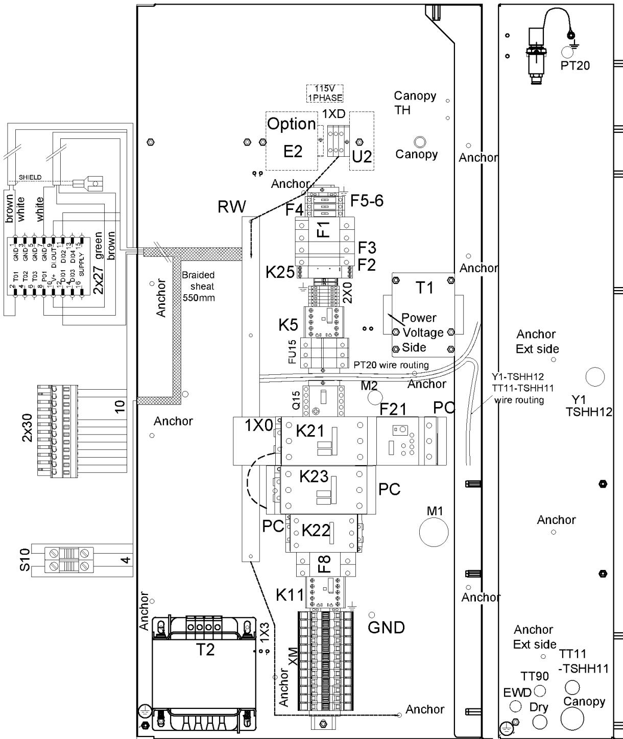
**39 - Cubicle components CPBg 20-34 - 200230460V - CRNSASME - With dryer - Gear driven**
