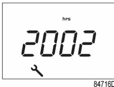
Example of running hours screen
