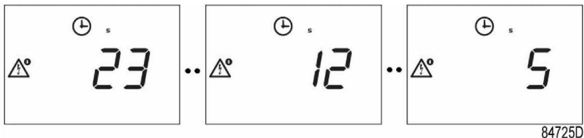
Example countdown delay time of automatic restart after power failure.
