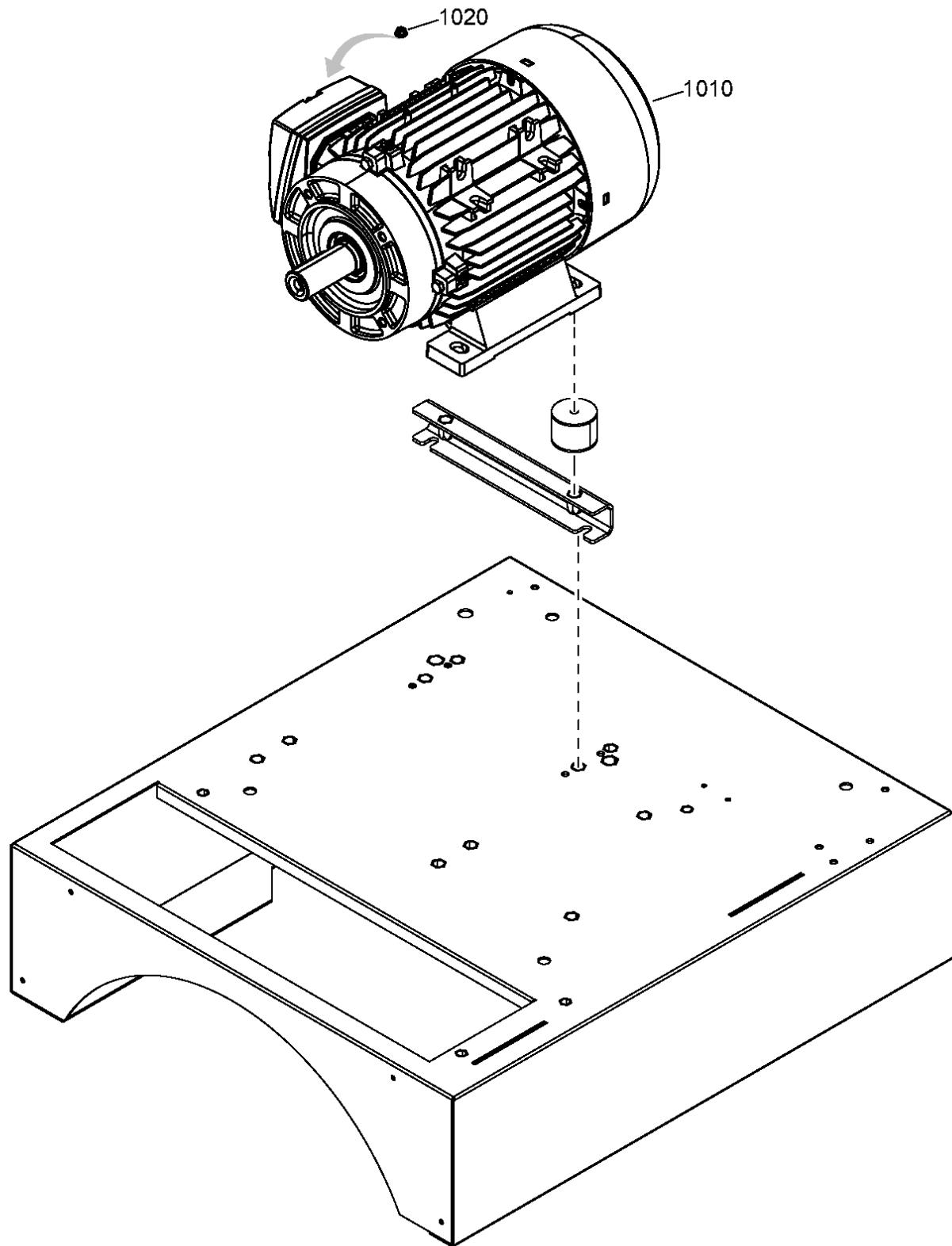
**3.7 - Motor (CPM 3, CPM 4, CPM 5.5) - 230V/50Hz - 3ph, (CPM 3, CPM 4) -**
