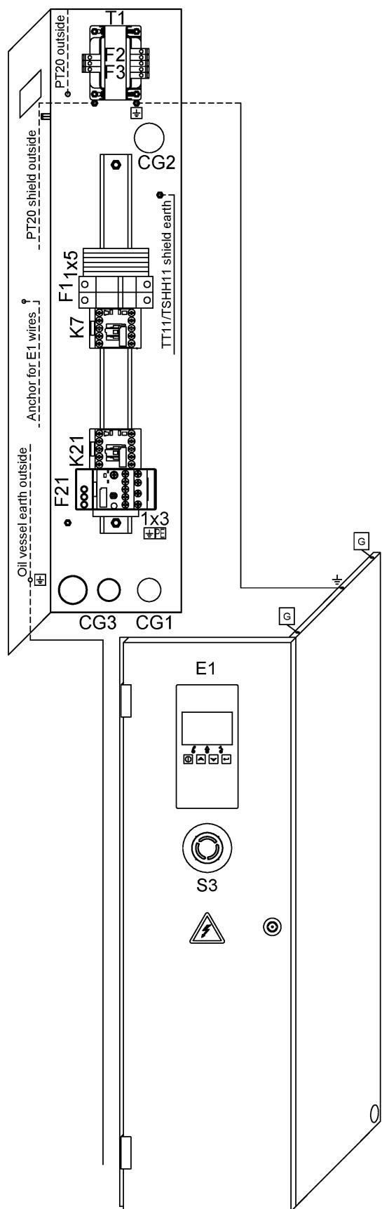
**18.4 - Cubicle components (CPM 3, CPM 4, CPM 5.5) - 400V/50Hz - 3ph - Basic control - DOL Starter**
