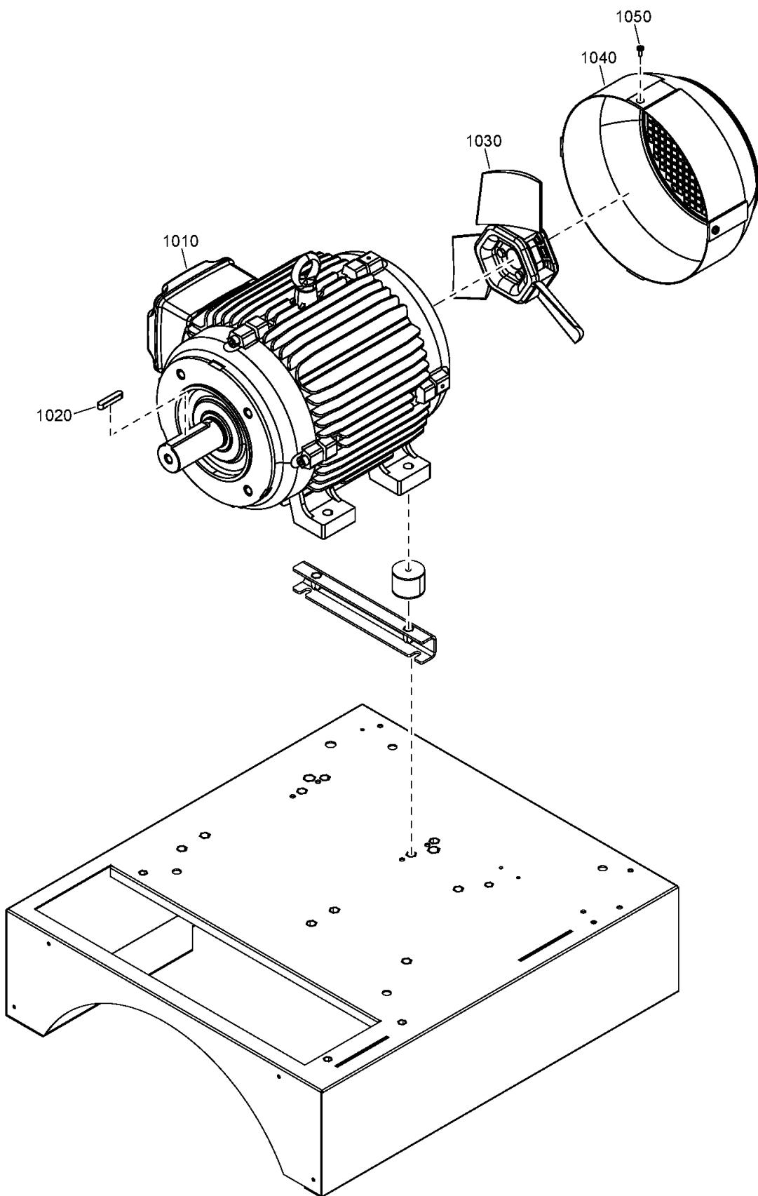
**3.9 - Motor CPM 7.5 - 230V-380V-440V/60Hz - 3ph, CPM 9 - (230V/50Hz, 230V-380V-440V/60Hz) - 3ph**
