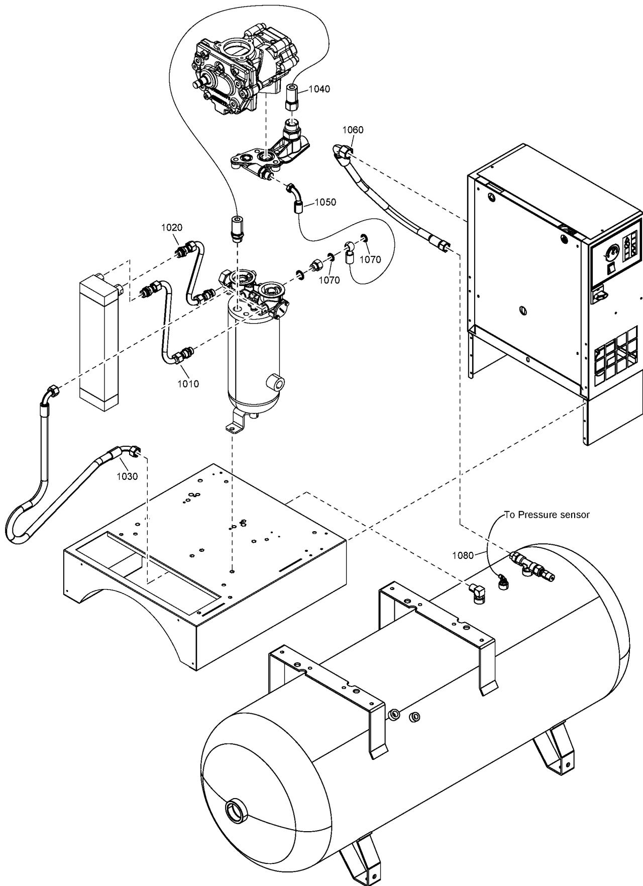
**13 - Air outlet 270L - Tank-mounted - With dryer**
