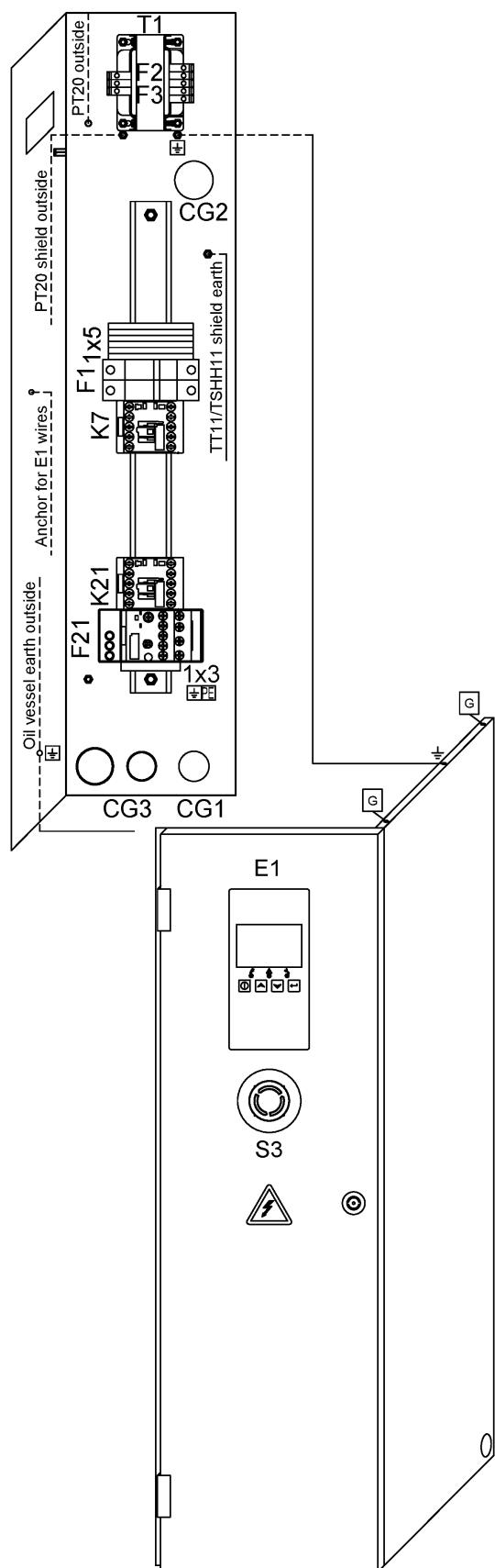
**18.5 - Cubicle components CPM 3, CPM 5.5 - 380V-440V/60Hz - 3ph - Basic control - DOL Starter**
