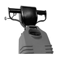
Now the machine can operate at full efficiency until all the detergent solution is out by turning the operating lever that drives all controls [G].
