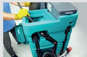
1. Take the machine to a suitable area for the disposal of waste water and turn it off. The brake will activate automatically.
