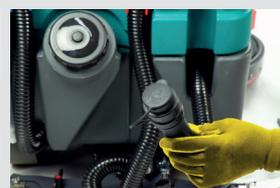
4. Inspect the brushes to make sure they are clean and in good condition. If the bristle length is close to the wear indicator (red color), replace the brush.
