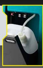
ADJUSTABLE DISTRIBUTION OF CLEANING SOLUTION UP TO 5 LEVELS, AND PROPORTIONAL TO SPEED OF MACHINE This allows for the complete control of detergent use, while providing the ability to increase or decrease the flow of cleaning solution, customizing the performance of the machine to the type of surface to be cleaned.
