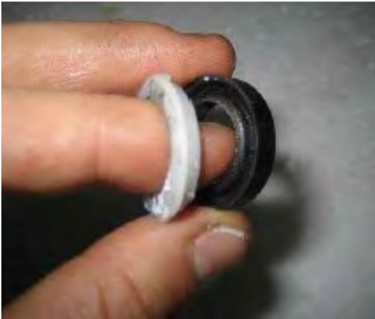
Assemble White & Black Packing and insert into pump
