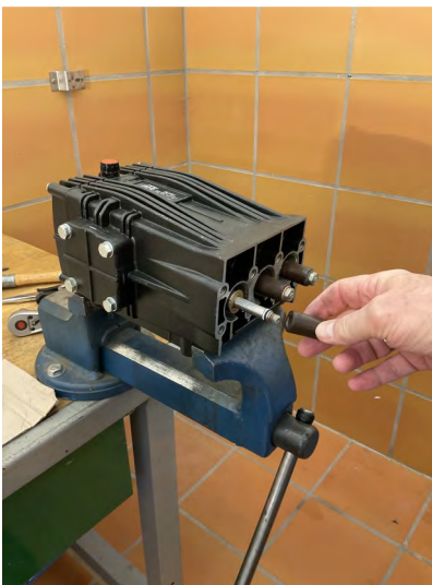
Grease O-ring with water resistant grease. Install ceramic piston on piston rod.
