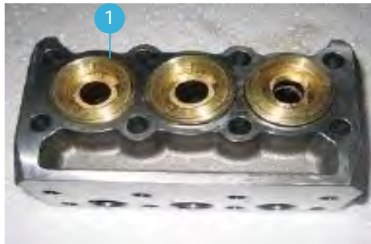
Insert the Pressure Ring (1) into the Pump Head, knock a few times with a mallet to compress the packing below
