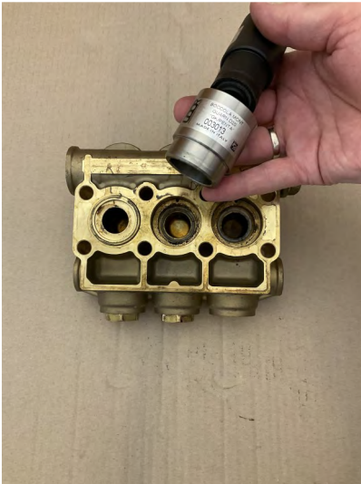
Install primary seal in special tool
