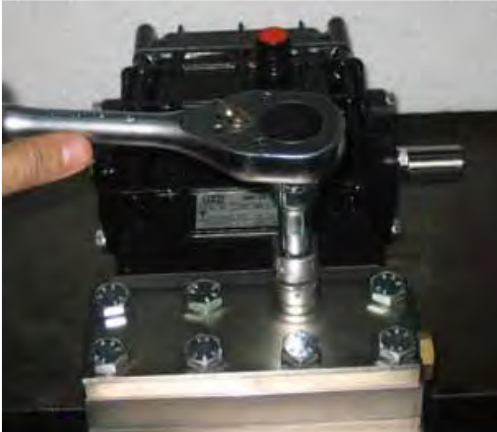
Remove the M10 bolts, and then remove the Outlet valve cover.
