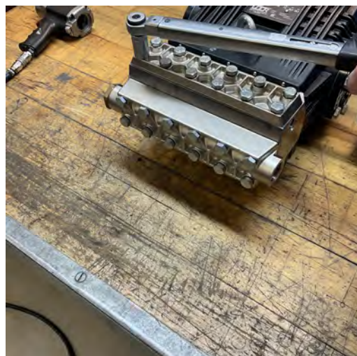
Mount the pressure valve cover and tighten with correct torque. (50Nm)
