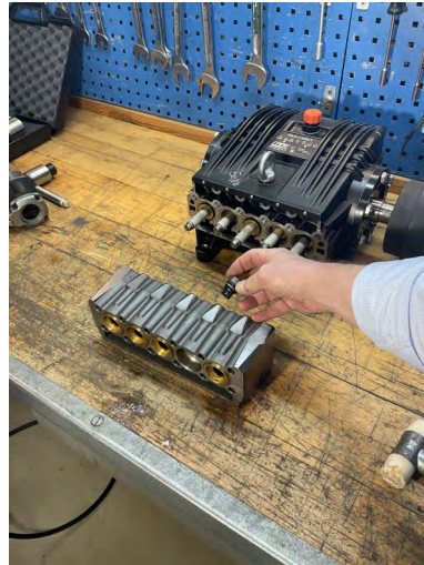
Suction valve dismounted. Remember to remove the spacer below the valve.
