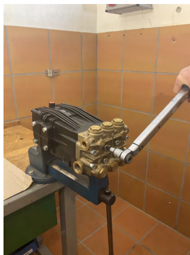
Install the cylinder head and tighten the 8 bolts with the specified torque.
