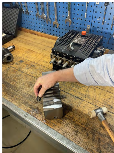
Secondary seal dismounted with the use of the special mandrel.
