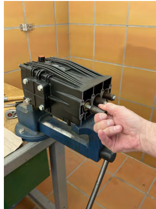
Pull out the ceramic piston.
