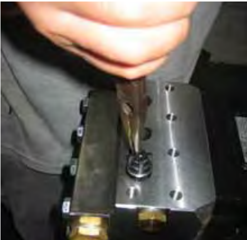
Pull out the valve using a set of pliers. Check the valves for damages, replace if needed.
