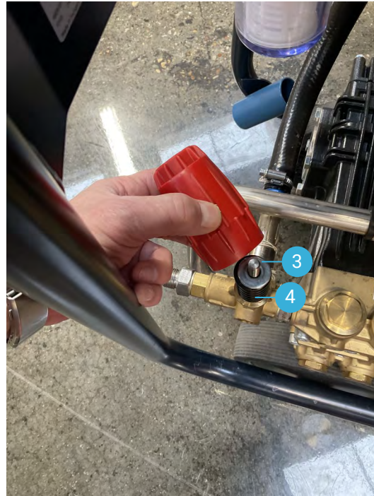
STEP 1 – Remove nut (1), handle (2), washer (3) and spring (4)
