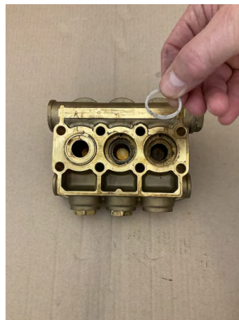
Install support ring for primary seal
