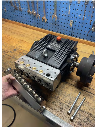
Lift off the manifold.
