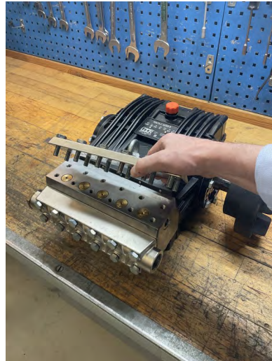
Lift off the cover plate
