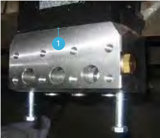
Mount the pump head. Push the pump head until there are no gab (1) between the crankshaft housing and pump head.
