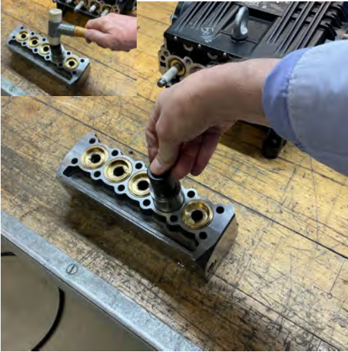
Assembly mandrel correct positioned in cylinder head. Push hard on the mandrel to mount the water seal. If needed knock on the mandrel with a plastic hammer.
