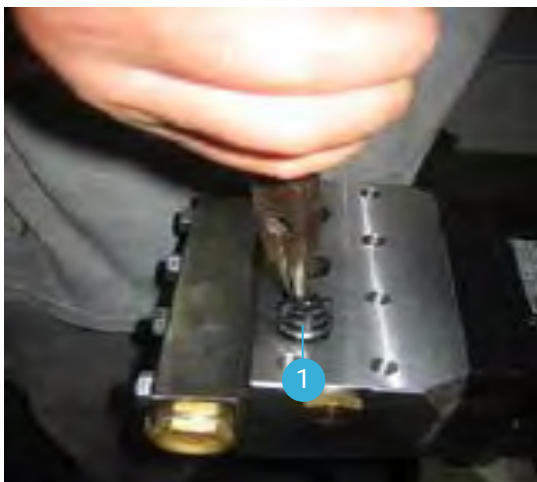
Mount the Valve and O-ring into the Pump Head
