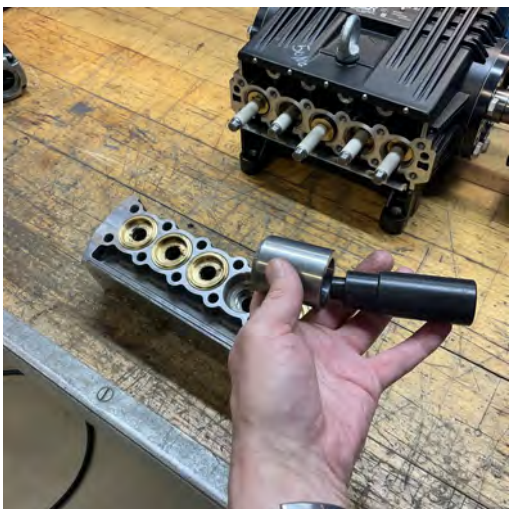
Special tool (assembly mandrel) for primary water seal.
