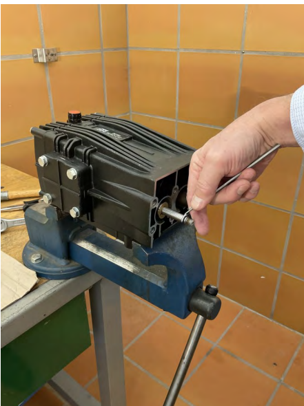
Carefully remove the back-up ring and the O-ring from the piston rod.
