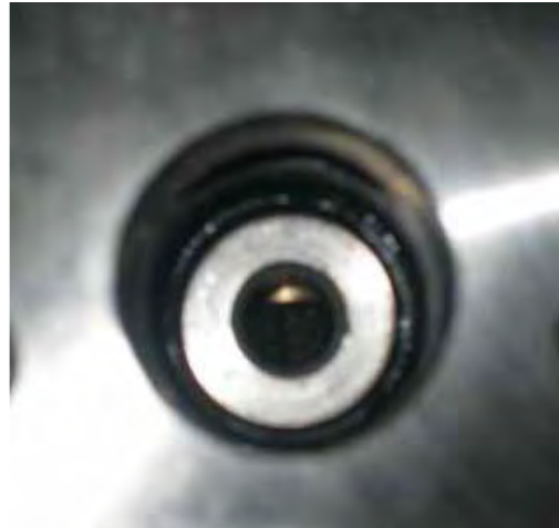
Use an O-ring picker tool to remove the O-ring below the valve.
