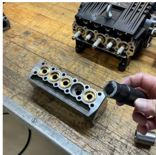
Seal mounted on mandrel
