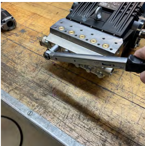
Mount the suction manifold and tighten with correct torque. (50Nm)
