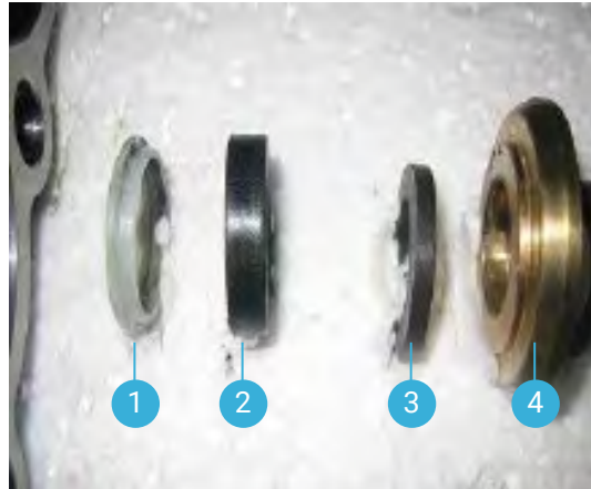
Mount the seals and back ring as shown above. Pay attention to the seal sequence from left to right, White (1), black (2), brown (3) and back ring (4).
