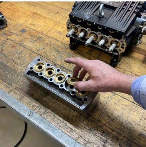
Mount the brass support ring
