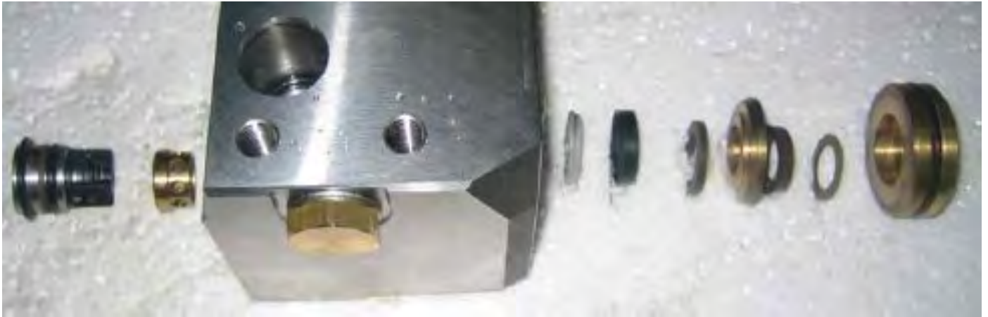
Disassembled view of pump head & manifold
