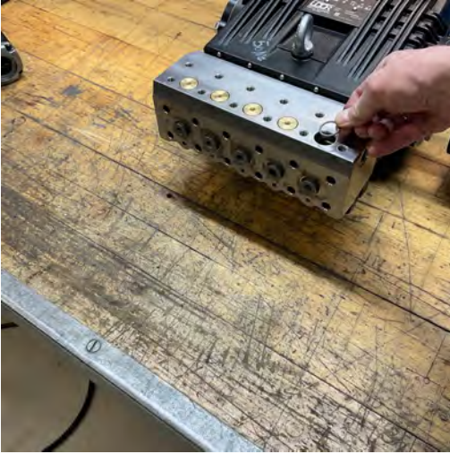
Installing the pressure valves. Remember to first mount the backup ring in the bottom of the hole.
