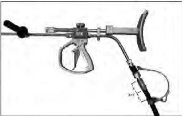
Correct mounting of connector safety device between hose and dump gun.
