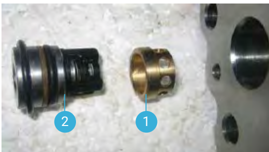
Turn the Pump Head over and insert the Diffuser (1). Note the orientation.
