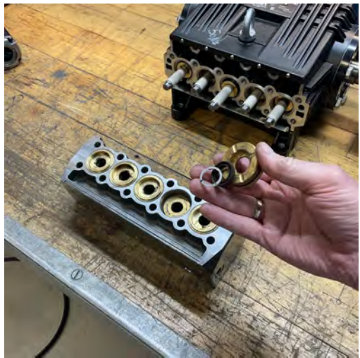
Secondary water seal position in thrust collar.
