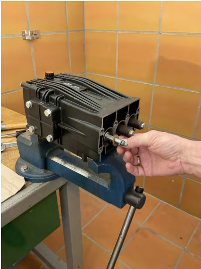
Install brass washer on piston rod.
