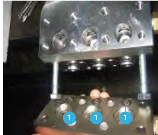
Mount the Manifold ensure that the cooling holes (1) are not blocked before assembling. Hand tighten the M10 bolts
