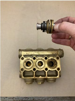
Primary and secondary water seals removed. IMPORTANT: make sure the support ring in the bottom of the water seal hole is removed.
