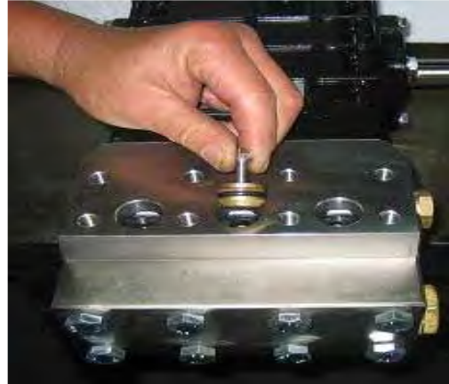
Insert an M6 screw and pull out the outlet valve cap.
