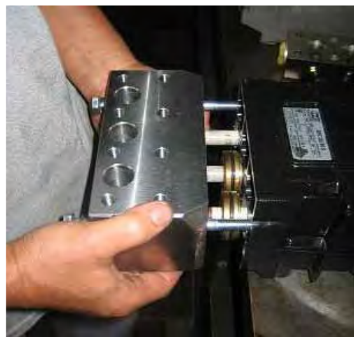
Remove the last 2 bolts for removing the manifold and pump head.
