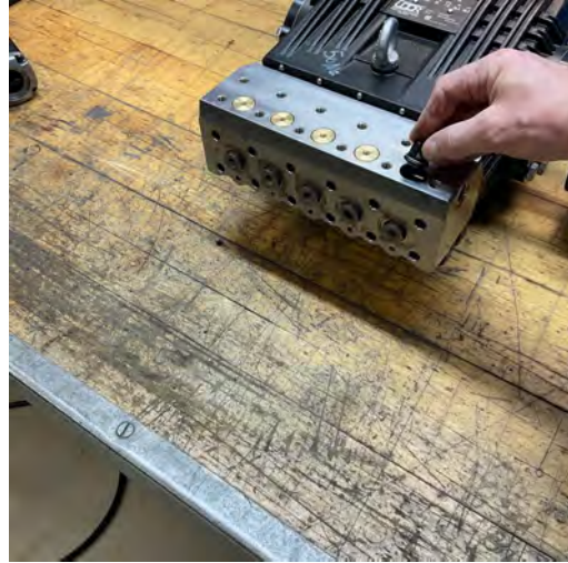
Mount the O-ring on the valve seat and lubricate with grease. Now push the valve all the way to the bottom of the hole.
