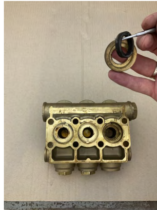
Remove the primary water seal from the brass ring. IMPORTANT: DO NOT make any scratches on the inside of the brass ring.
