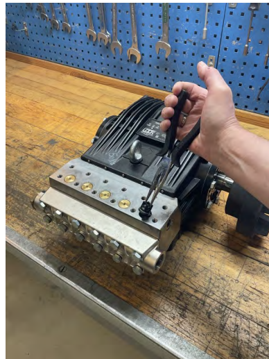
With a pair of pliers lift up the pressure valve. Make sure you also get the seat O-ring in the bottom removed
