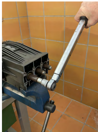
Tighten piston nut with the specified torque.
