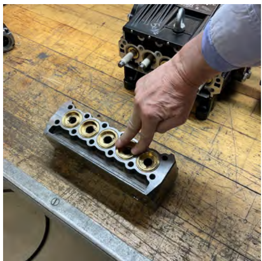
Push the thrust collar all the way to the bottom of the hole. Make sure all 5 are aligned.
