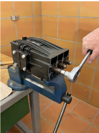
Loosen and dismount the 8 mm nut holding the ceramic piston
