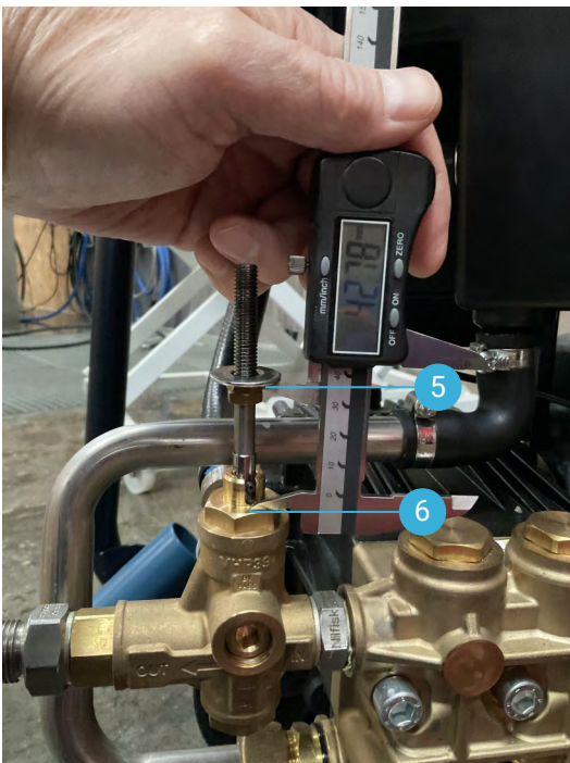
STEP 2 – Adjust the distance between lower side of washer (5) and pos. (6) to 42,8 mm
