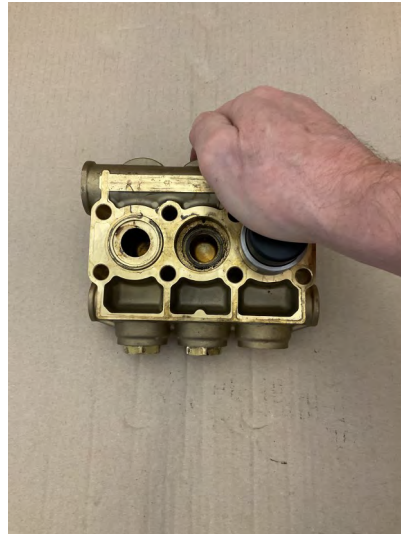
Install metal part in cylinder head, and push hard on plastic part to install primary seal in cylinder head.
