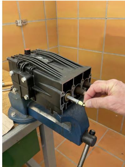
Install back-up ring and O-ring on piston rod. Protect the O-ring from damages from the threads when installing. Here is used a small piece from a post-it block.
