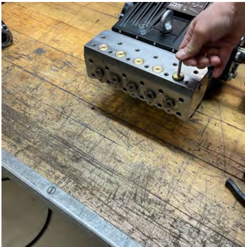
Grease spacer O-ring, and push the spacer all the way down. A 5 mm bolt can be used.
