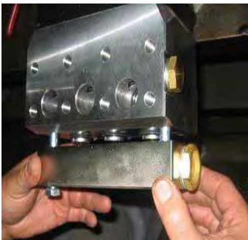
Loosen and remove the 10 mm bolts, except 2. Now remove the last 2 bolts
