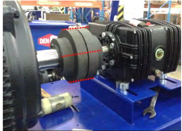
Shim used to correct any height misalignment
