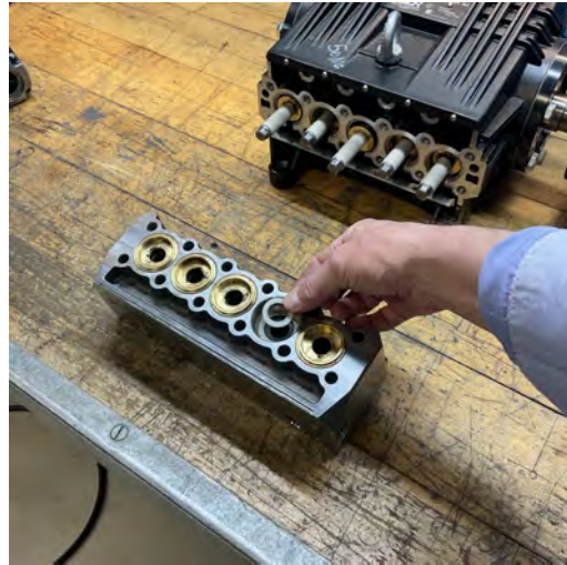
Mount the backup ring on top of the seal.
