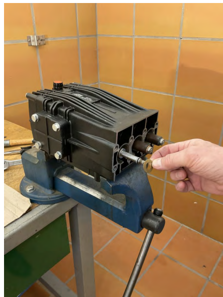
Remove the brass washers from the piston rod.
