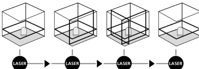
! The transport restraint must be released for horizontal and vertical levelling. The laser lines flash and a signal sounds as soon as the device is outside the automatic levelling range of 3.5°. Position the device such that it is within the levelling range.
