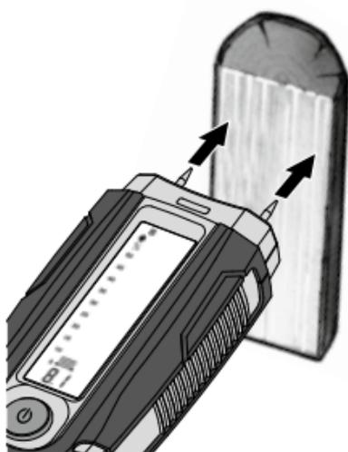
The location to be measured should be untreated, free of knots, dirt and resin. Measurements should not be made on the end faces of wood because these areas dry particularly quickly such that they produce incorrect measurement results.
