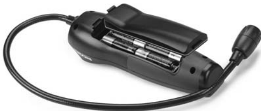
Figure 4 – Removing Battery Compartment Cover
