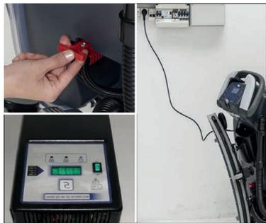
19. Charge the batteries: Connect the battery charger cable to the electrical socket.
