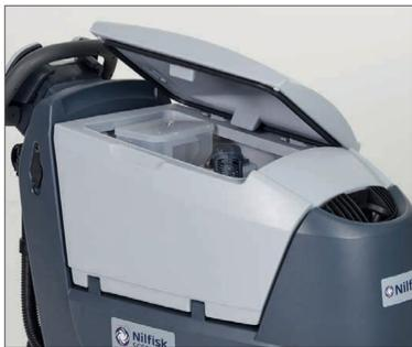
20. Park the machine with the recovery tank cover open.
