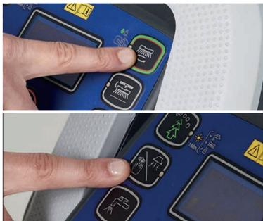
10. If necessary press the extra pressure function (hold for one second). If necessary press the silent mode button for extra low sound level.
