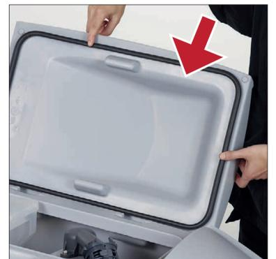
4 Check the lid gasket is in good and working condition and sealing when lid is closed.
