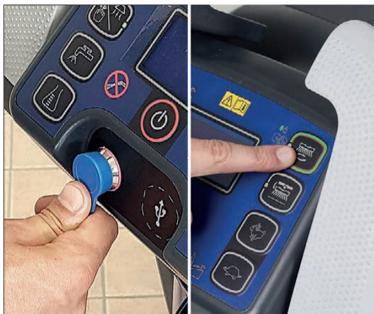
6. Place the user key in the key reader, then start the machine by pressing the One-Touch button. To engage the brush, slightly press the drive paddle and then release it.
