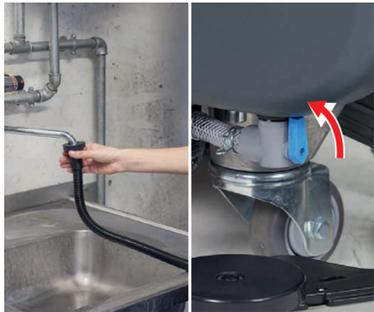
2. Fill the tank with a clean water. The clean water temperature must not exceed 40 °C. Make sure the solution valve under the machine is open.
