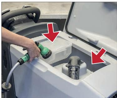
14. Empty the debris tray and clean/wash the recovery tank inside.
