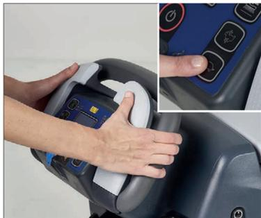
8. Push forward the drive paddle to start cleaning. Adjust maximum speed by the speed regulation buttons.
