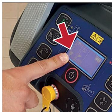
2 Check if there isn't any brush motor overload "WARNING ALARM F2" on the display.
