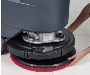
5. Place the brush or the pad-holder under the deck. Use the appropriate brush to clean the floor.
