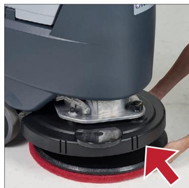
3 Check if the brush are correctly installed and not worn out or if there are external materials avoiding brush rotating.
