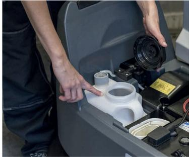
3. Fill the EcoFlex tank with a detergent suitable for cleaning machines (highly concentrated and low foaming detergent).
