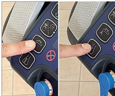
9. To change the solution flow level push forward the solution button and change flow level according to the cleaning performance and application.
